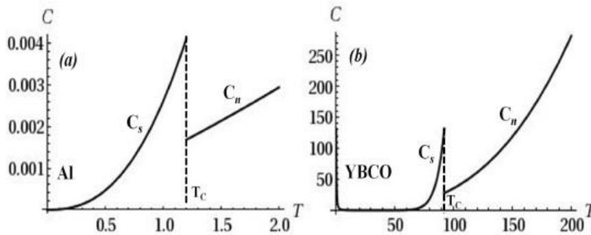
**FIG 2.** Specific heat of Al and YBCO; C is in J/mol-K.
