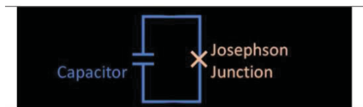
FIG 2. Capacitor with Josephson junction.
