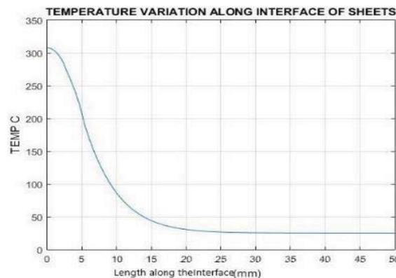
**FIG 10.** Temperature variation along the interface.
