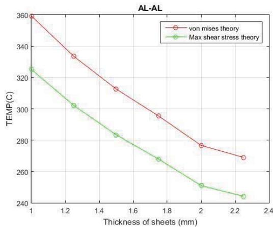
FIG 5. Thickness vs temperature for Al-Al pair.
