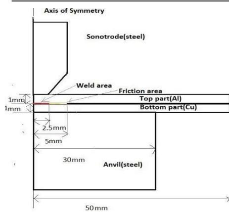
FIG 3. Axisymmetric model.
