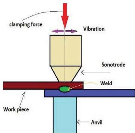
FIG 1. Ultrasonic welding.
