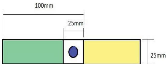
FIG 2. Standard specimen.
