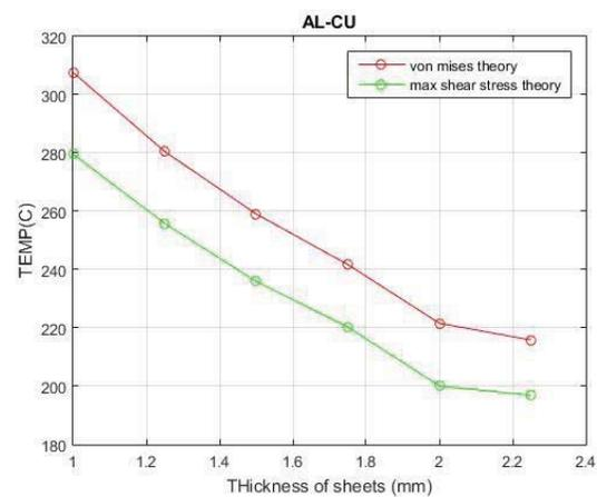
FIG 6 Thickness vs temperature for Al-Cu pair.
