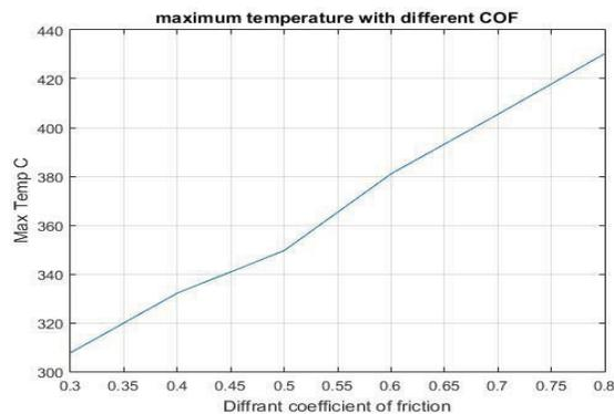
FIG 13. Temperature variation with different coefficient of friction.
