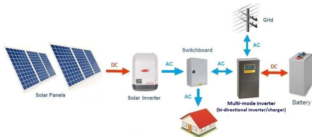
FIG. 4. Hybrid solar power plant
